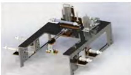
Automatic clamping heat-staking machine for holding pieces with hot-riveted joints during assembly
