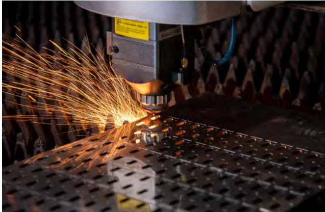
● Laser cutting using a CNC fibre laser cutting machine
